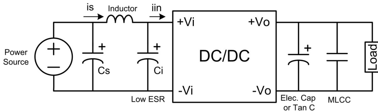
Measured input reflected-ripple current with a simulated source Inductance. Capacitor( $C_s$ ) offset possible Power source impedance
